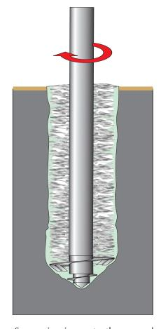
Suspension is constantly pumped to the mixing tool while lowering to the required depth.
