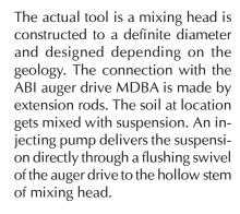
Since mixing is actually achieved during lowering and withdrawing of the tooling, one speaks of a two step method. The load-bearing capacity and firmness of the column are determined by the amount of injected cement suspension and consistent stirring.
