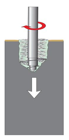
Lowering the mixing tool into the soil with 100 – 200 rpm. A substantial amount of soil gets mixed with under pressure injected suspension.
